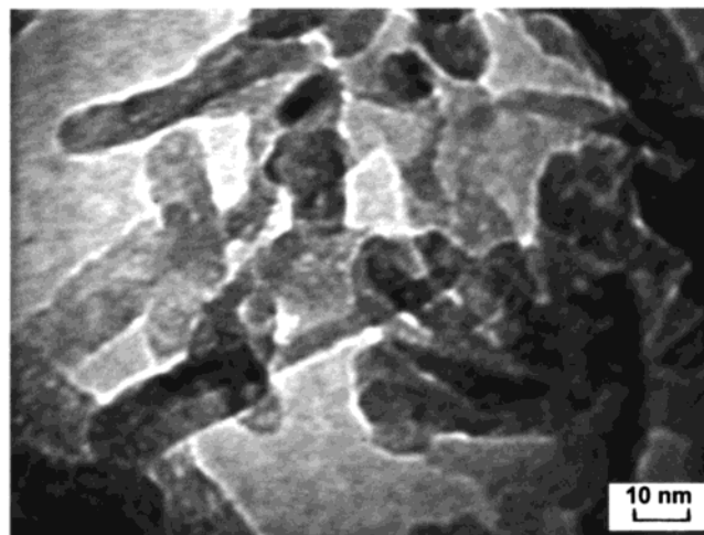
Figure 4. TEM micrograph of powder prepared in the presence of Brij-30 with (Ca/P)r = 1.65 after 7 days of aging.
